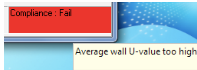
Figure 16.2: Tool tip showing the primary cause of failure
