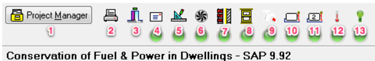
Figure 18.3: The SAP toolbar: 1 – Return to Project Manager . 2 – Print . 3 – Exit JPA Designer. 4 – Project information (section 18.5). 5 – Dimensions tab (chapter 19). 6 – Ventilation tab (chapter 20). 7 – Walls, roofs and floors tab (chapter 21). 8 – Openings tab (chapter 22). 9 – Hot water tab (chapter 23). 10 – Primary heating tab (chapter 24). 11 – Secondary heating tab – (chapter 25). 12 – Overheating tab (chapter 26). 13 – Photovoltaic and alternative technologies tab (chapter 28).
