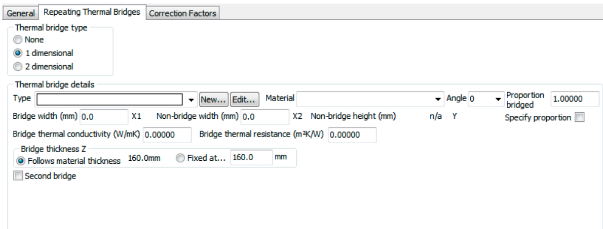
Figure 7.5: The Repeating Thermal Bridges tab
